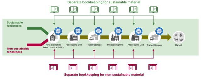
Fig 4: Simplified example for mass balancing in a supply chain for biofuels
